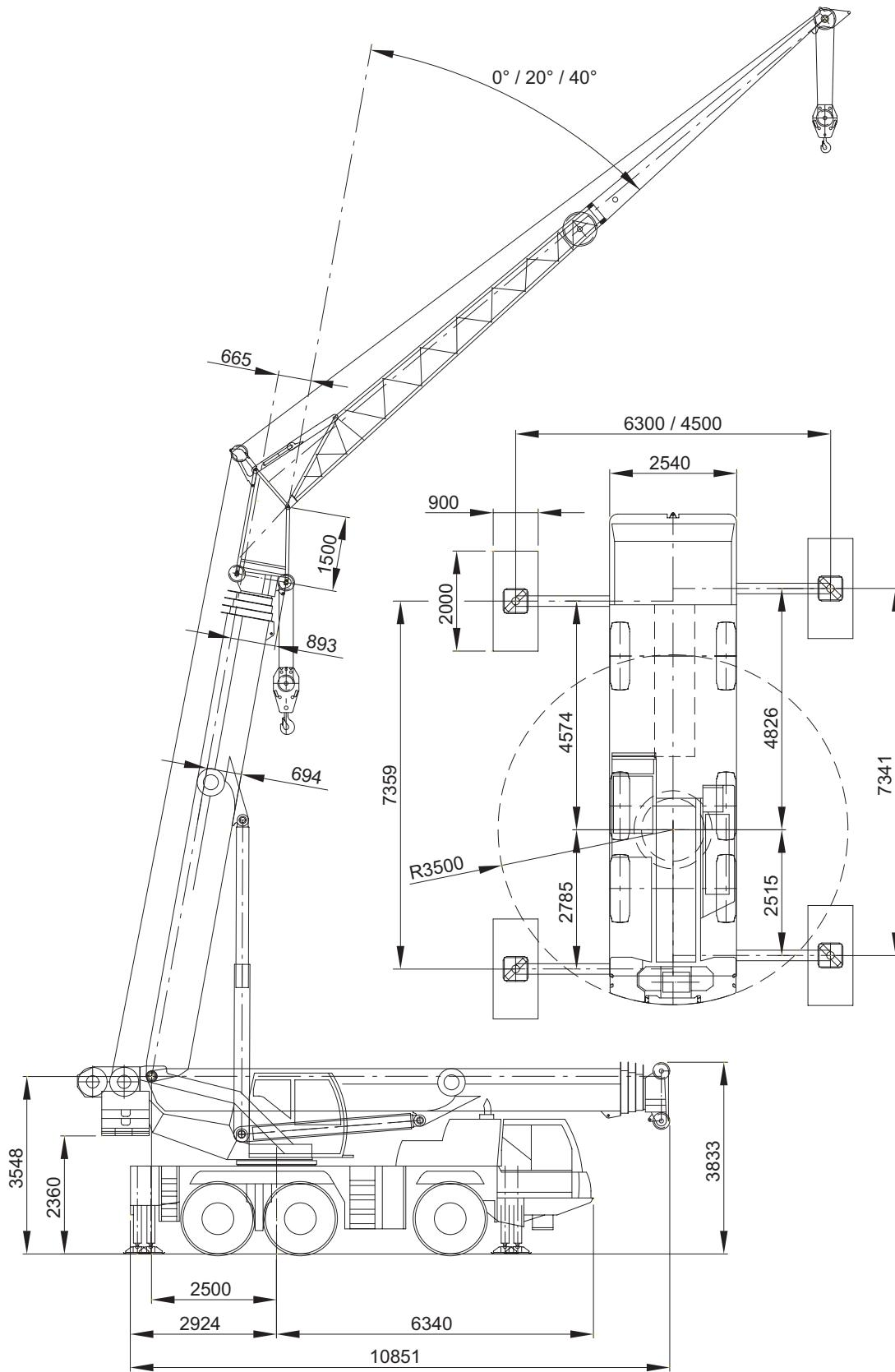
Dimensions are in millimeters.
